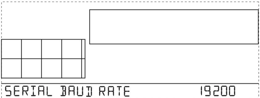
Use the up (+) and down (-) arrows to change the Baud Rate setting, if needed. Press and hold DONE to return the console to the current weather mode.
