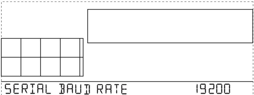
The Baud Rate setting on the console must be same as that set in the WeatherLink software. Use the up (+) and down arrows (-) to change the Baud Rate setting, if needed. Press and hold DONE to return the console to the current weather mode.
