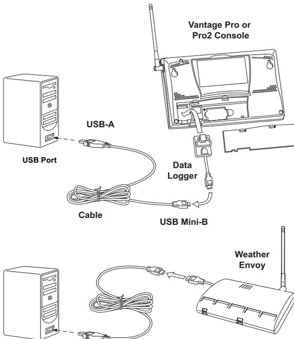
6. Insert the USB - Mini B connector on the USB connector of the USB data logger. The connection between the console and the computer can be extended up to 16' (5 m) using a USB-to-USB connector cable.
