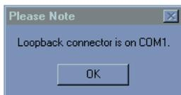
The correct COM port is automatically selected in the **Communications Port** dialog box. If the loopback connector is not found on any COM port, your serial port may not be working. If a connection still does not exist or if the loopback test identifies the same serial port you have selected, eliminate the following possibilities:
